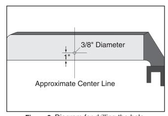
Figure 2. Diagram for drilling the hole.
